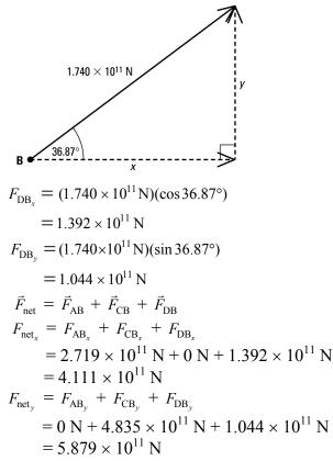
Use trigonometry to determine the net electrostatic force on charge B, as shown in the following diagram.
